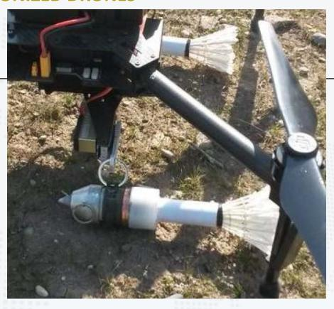
Quadcopter modified with an improvised releasing system and modified 40mm grenade projectile / equipped with an dual releasing system and two attached improvised bomblets
