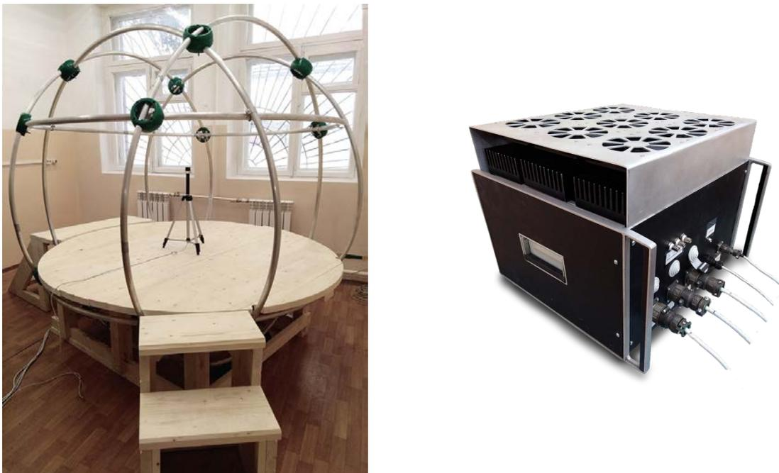
**Figure 3.** Automated stand for reproducing magnetic field: on the left – a three-component coil system of Helmholtz coils, on the right – a functional block.
