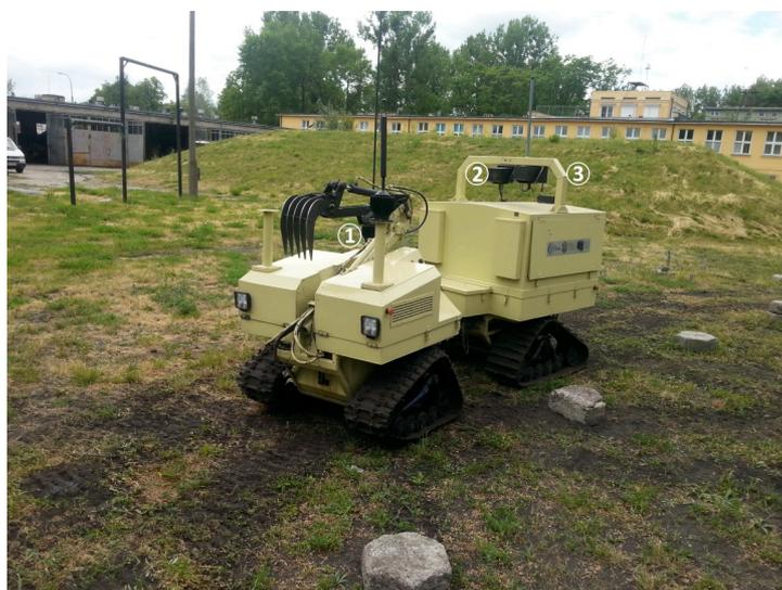
Figure 1 Dromader robot. Robot's cameras marked as 1,2,3
